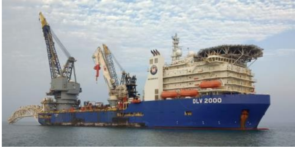
Pipeline Installation Vessel: DLV2000
