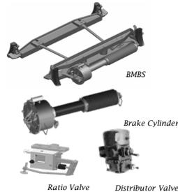
Bogie-mounted brake system
