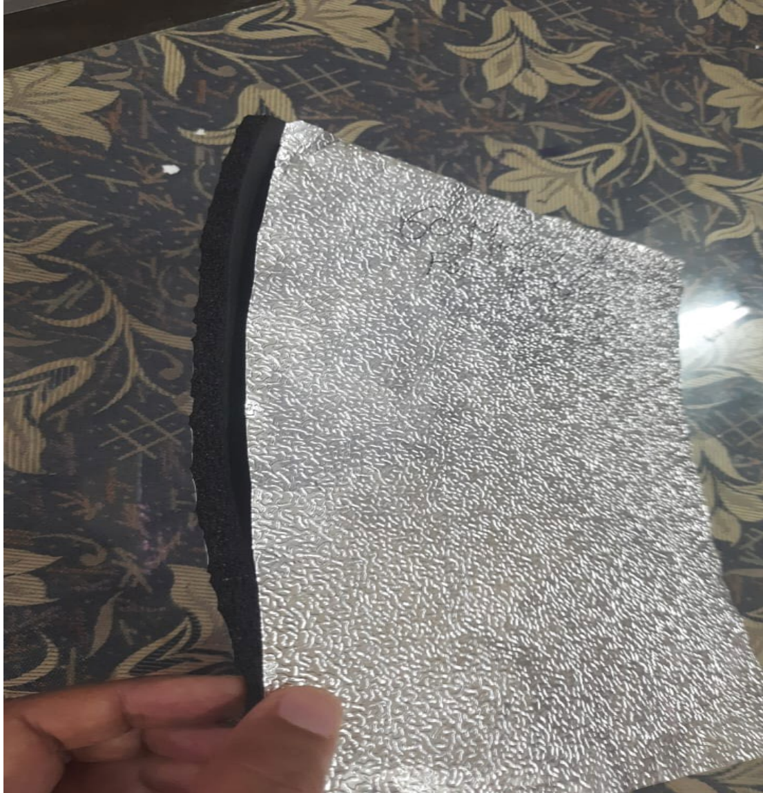
60 Micron Aluminum with NBR Foam
