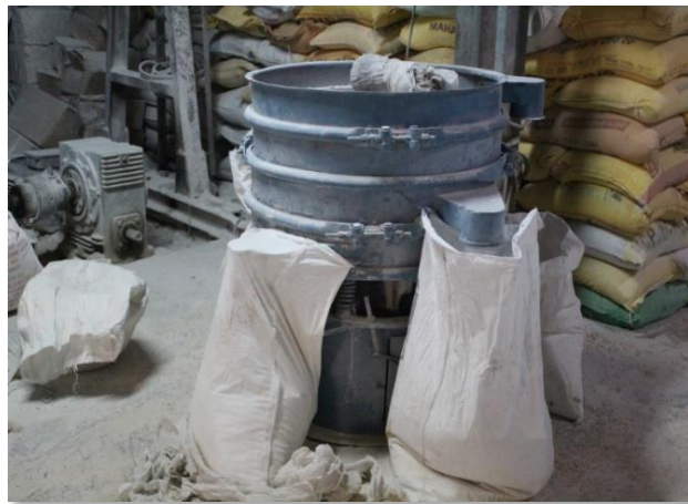
Raw material sieving –(40 fine to 4#) – to remove lumps from the raw material
