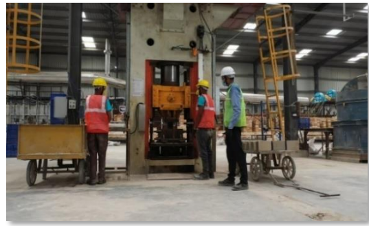
Press machine for making the bricks
