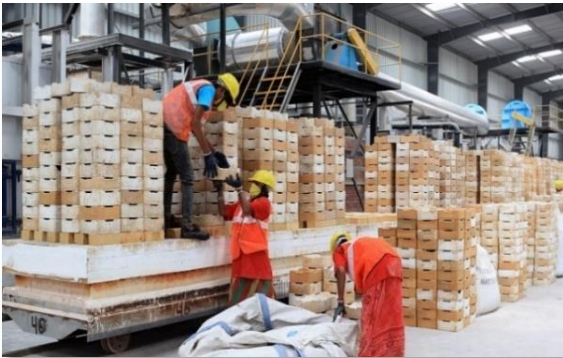
Loading the material into the tunnel kiln for firing
