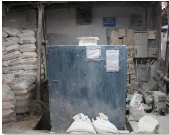
Ball mill-2 – for crushing raw material into fine powder
