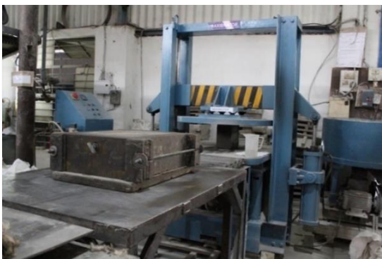
Maxibrator-for complicated production- intricate shapes of any size are made using our maxibrator machine wherein the mould is pressed in the maxibrator machine
