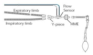
FIGURE 3-1 Installing the Flow Sensor
