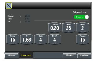
Figure 6-19 All parameters in SIMV-PC mode
