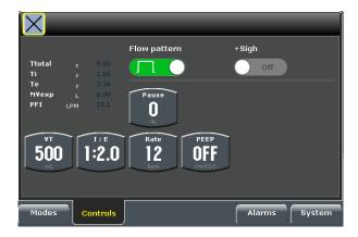
FIGURE 6-4 All parameters in VCV mode
