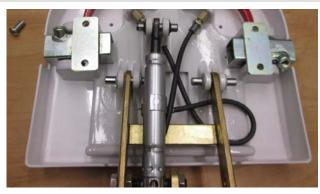
Apply a thread locker such as Loctite® 242 to screw. Repeat with three remaining screws.
