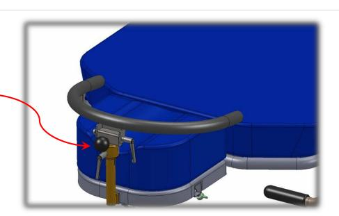
Rotate wrist rest slope adjustment knob until desired position is achieved.
