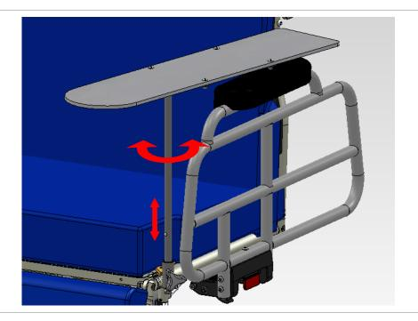
3) Rotate adjustment knob clockwise to lock armboard in desired position.
