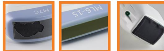
**Any damage to the transducer that would allow fluid to infiltrate the transducers internal components is an AUTOMATIC FAILURE. The transducer should be removed immediately from service.**
