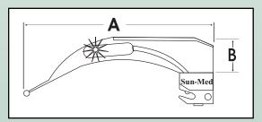
All above blades are made from 303/304 surgical stainless steel and are provided with 4mm, replaceable fiber optic bundles.
