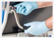
Lowering the Push Bar Grasp the push bar handle while pulling out the Red release knob and lower the push bar.
