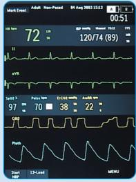
A typical monitoring view shows some basic patient information, the date, time and battery status. Next are the numerics and waveforms. The bottom half of the screen shows additional monitoring numerics followed by their waveforms, and soft keys for customizing the display, setting and responding to alarms, and selecting parameters to view additional monitoring data.
