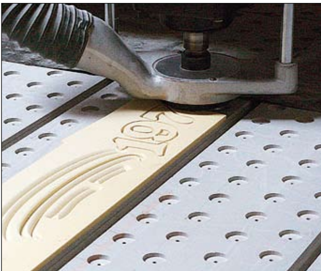
Using thin material is key when forming over a shape. Here I am cutting the letters and ribbing out of 1/4" Sign Foam. A round-over bit is used on the ribbing along with simple male cuts.
