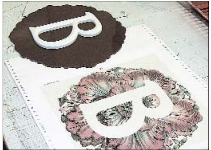
The PVC (polyvinyl chloride) letter is routed with a prismatic profile and attached to an acrylic back. I printed a rosette on the Gerber EDGE and applied it to the acrylic. A letter this ornate would be best used as a short word such as "Boutique".
