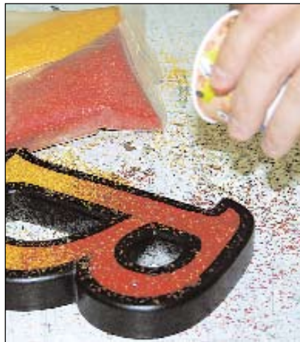
The PVC (polyvinyl chloride) letter is routed with a prismatic profile and attached to an acrylic back. I printed a rosette on the Gerber EDGE and applied it to the acrylic. A letter this ornate would be best used as a short word such as "Boutique".
