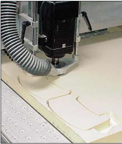
The banners are cut out on the router table. A clean-out path is dedicated to the area where the banner folds around at a depth of 1 1/2".
