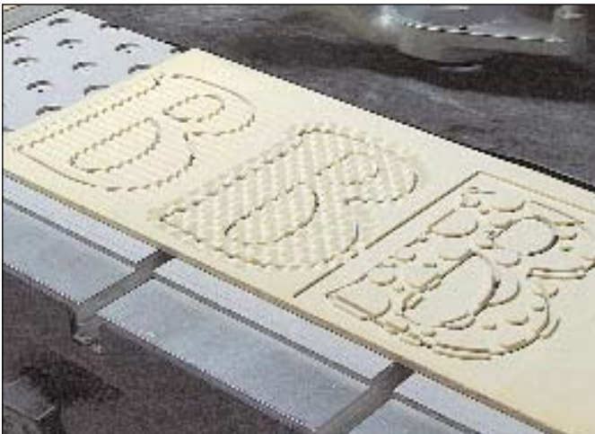
I included a box around the circles so as to run the clean-out necessary to create this style of texture or pattern.
