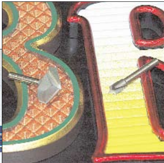
(Above) A close-up of the router bits used to shape the textures. I placed each bit on to the texture that they created.
