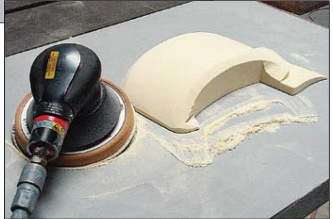
A pneumatic palm sander suited with 40-grit sandpaper makes quick work of forming the needed shape.
