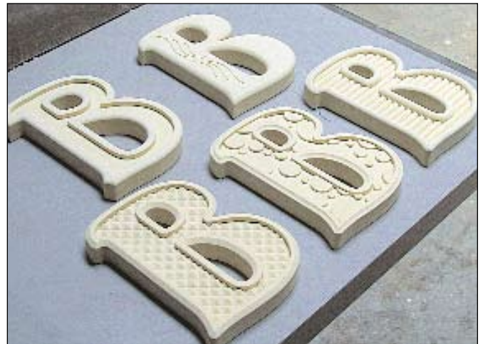
The inlays are fitted to the corresponding letter. I used an inlay tolerance of .012 for this run and after primer and paint it was a tight squeeze.
