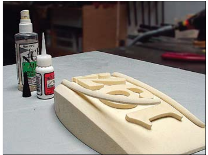
The cyanoacrylate glue and accelerator are shown here. Because of its watery consistency it's best to work your way across each piece slowly from one end to the other in a "tack weld" fashion.
