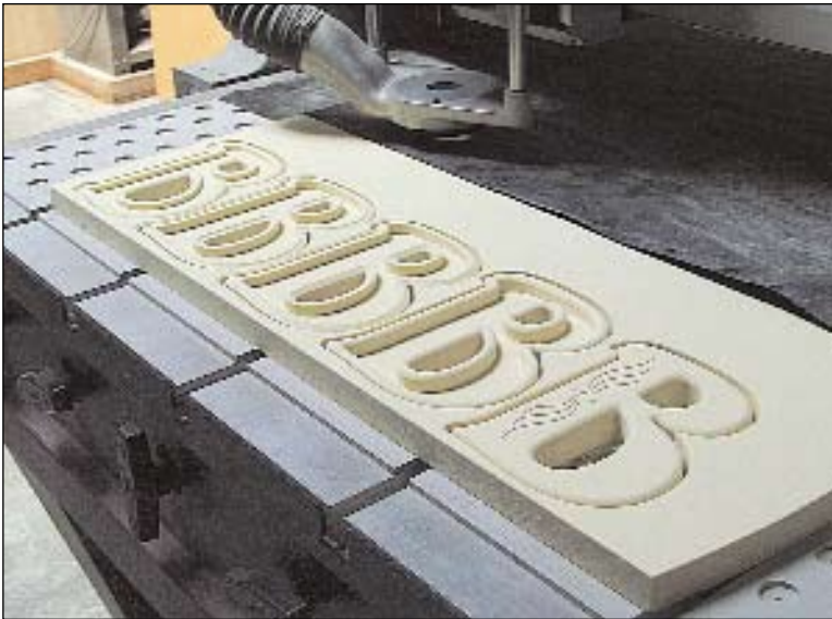
Using 15-lb. Sign Foam each "B" is cut out and receives a different edge profile. Using the inlay feature, four of the letters are assigned a cleanout path to remove the material.
