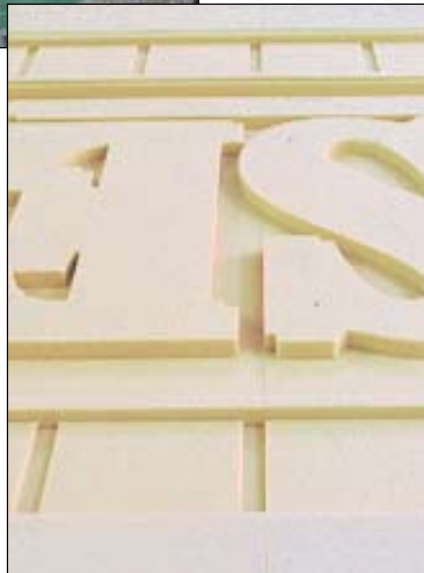
On a completely different job notice how I chose to run the seam down the edge of the paneled grooves. The sign will also receive appliquéd letters and bamboo border treatments to further hide the seam.
