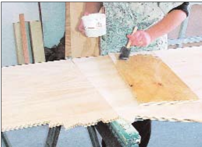
Working on the backside of the sign, epoxy is spread on to this precut seam plate that when applied will straddle the seam. 15 lb. Sign Foam is used in these examples, but the techniques will apply to other densities and brands of HDU.
