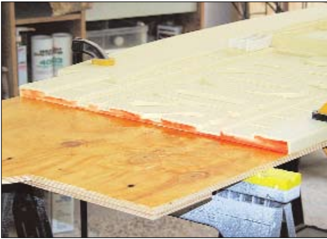
The first piece is clamped into position. This allows us to apply pressure to close the seam tightly with the second piece (we added color to the epoxy to better illustrate how we intentionally stay away from the surface).
