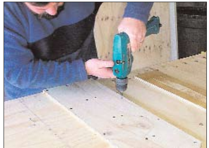
The plate is carefully screwed down to give this sign its length and strength. Extra plates are attached to the back to keep the sign flat when installed.
