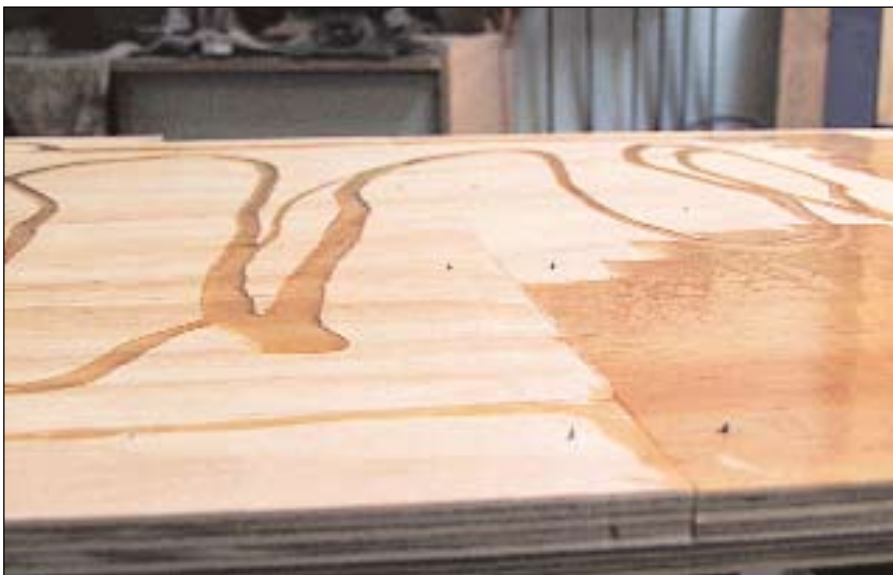
After the backing is together we flip it over so the face is up. Epoxy resin is poured over the entire surface and spread evenly with a roller.
