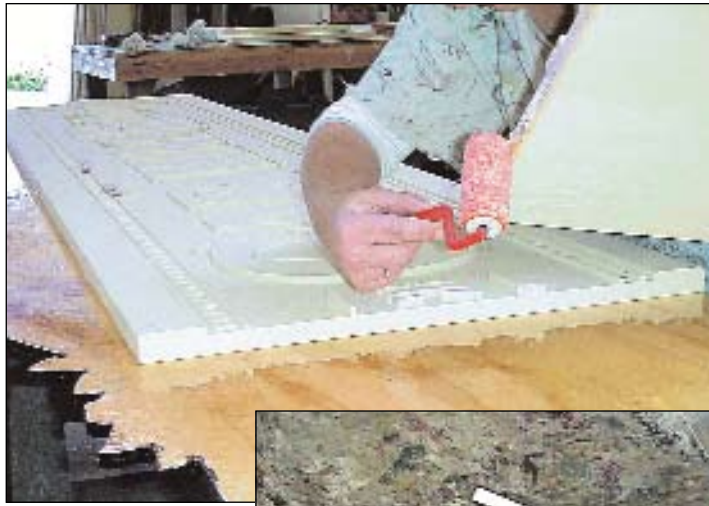
The HDU is laid into the epoxy bath. One end is coated with epoxy while taking care not to cover the surface edge. This will eliminate any excess from oozing out onto the face.
