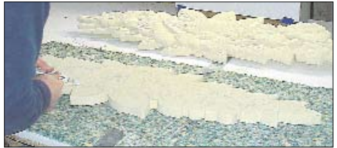
Here I am shaping the HDU to create the floral design. I use a lamp at a low level to help me see better and make faster work of this process.
