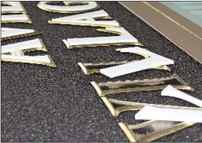
Black smaltz background housing a gold leaf outline of the letters. A 1/4" white acrylic letter was glued into the inlay using silicone adhesive.
