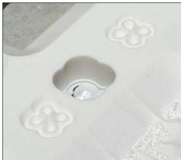
The stamp is tooled using a solid surface acrylic material. The cutting depth was adjusted for each test until I was satisfied. In this case the middle profile was preferred.
