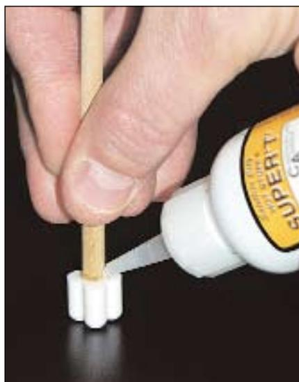
A wood dowel was attached to the stamp using cyanoacrylate glue and cut to a comfortable length to work with.
