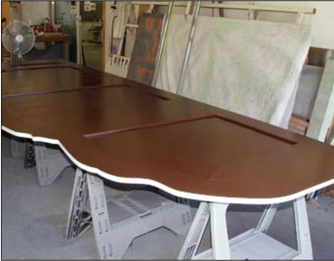
Using the router we cut a backer out of 3/4" marine plywood. The edge was reinforced as well as the areas where the sign will meet the 3" pipes during installation. It is easier to paint the back first and this method has become standard practice in our shop.
