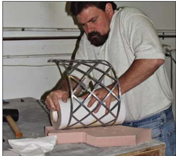
I shaped a large groove in a piece of scrap urethane to help me create the circle needed for the diamond cut-out rectangle. A heavy roll of sandblast resist aided in this hand-forming technique.
