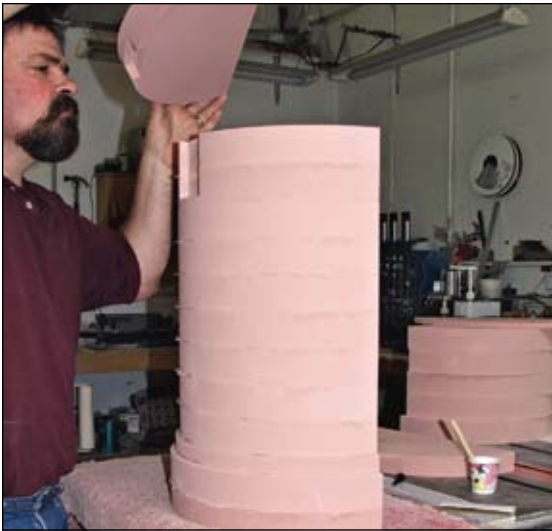
The main body of the lighthouse was created using 20 pre-cut urethane half circles. These were glued together with epoxy and tack welded in place using cyanoacrylate glue.
