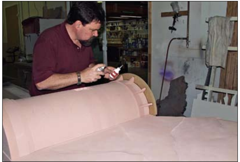
The catwalk surround was cut from 1" Extrite making it nice and durable. The photo shows me gluing the gussets in place.
