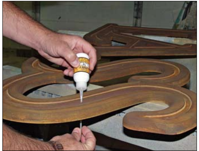
Quarter-inch all-thread is glued to the Sintra with cyanoacrylate glue.
