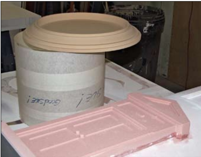
Here we see some of the parts created for the lighthouse. The doorway was cut on the router and glued to the main body. The 1/8" clear acrylic cylinder was masked to keep from scratching and cut to the right length with a band saw. Also, we see the bottom piece of the top (roof) this was cut with the router as well.
