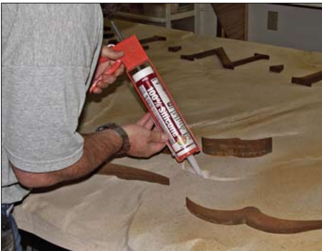
The pre-cut and rusted elements are secured into the inlaid areas with silicone adhesive. The close-up shows the different edge heights of the letters making for a solid appearance.
