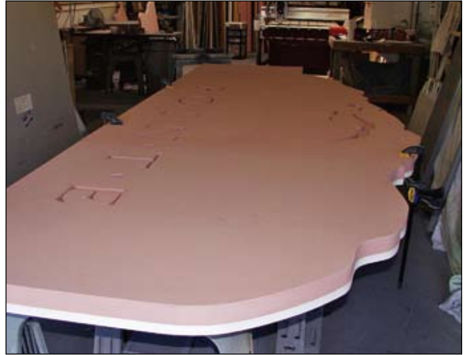
Two-inch SignFoam (10-lb.) has been router cut and epoxy glued to the backer.
