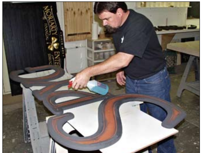
The 1/2" Sintra letter pads have been pre-painted with an iron paint and allowed to dry overnight. This photo shows me spraying the acid on the gray iron to turn it into rust.
