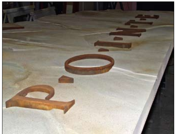
The pre-cut and rusted elements are secured into the inlaid areas with silicone adhesive. The close-up shows the different edge heights of the letters making for a solid appearance.
