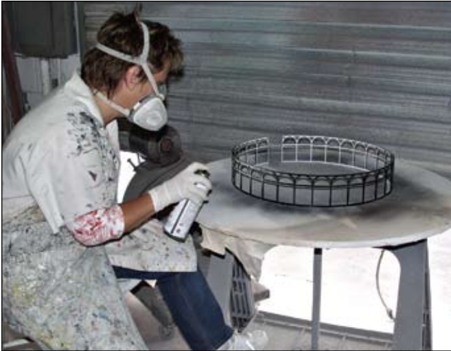
The Dibond handrail gets a black coat of paint. I gently hand rolled the handrail around the acrylic cylinder to get the shape that I needed.
