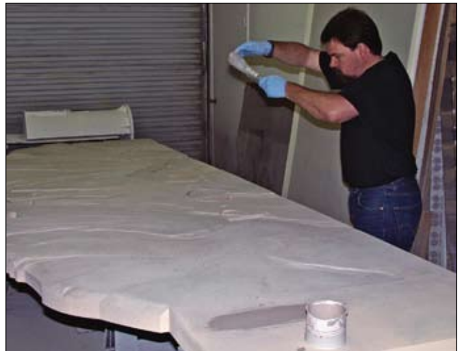
I painted the slab with three values of stone colors. Here I am spattering the pore structure with an old brush using some light and darker values. I finished off the slab with a taste of iron oxide (rust).
