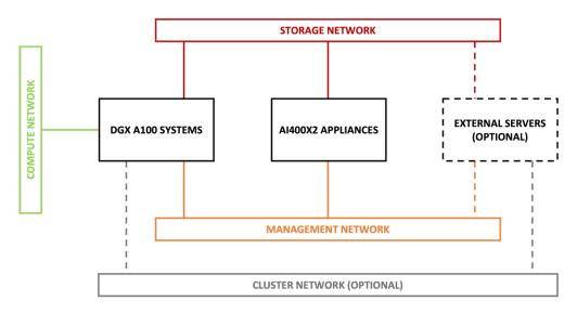
Figure 8. Overview of the DGX POD network architecture.
