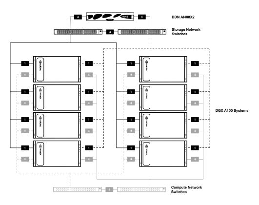
Figure 18. Test environment with eight DGX A100 system and one Al400X2 (management network not shown).
