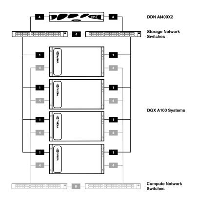
Figure 13. DDN A<sup>3</sup>I POD reference architecture with four DGX A100 systems (management network not shown).
