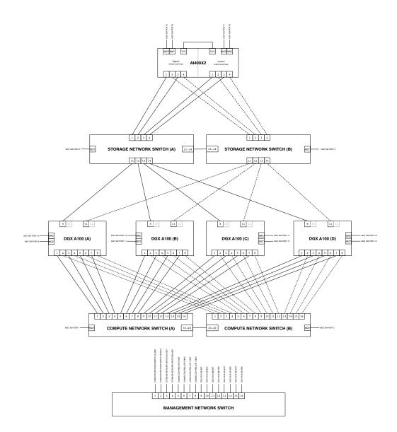
Figure 14. DDN A<sup>3</sup>I POD network diagram with four DGX A100 systems.
