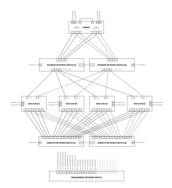
Figure 16. DDN A<sup>3</sup>I POD network diagram with eight DGX A100 systems (A-D).
