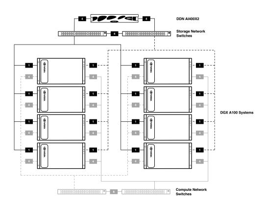
Figure 15. DDN A<sup>3</sup>I POD reference architecture with eight DGX A100 systems (management network not shown).
