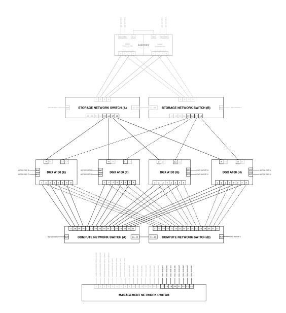
Figure 17. DDN A<sup>3</sup>I POD network diagram with eight DGX A100 systems (E-G).
