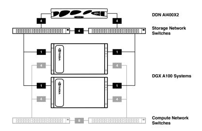
Figure 11. DDN A<sup>3</sup>I POD reference architecture with two DGX A100 systems (management network not shown).
