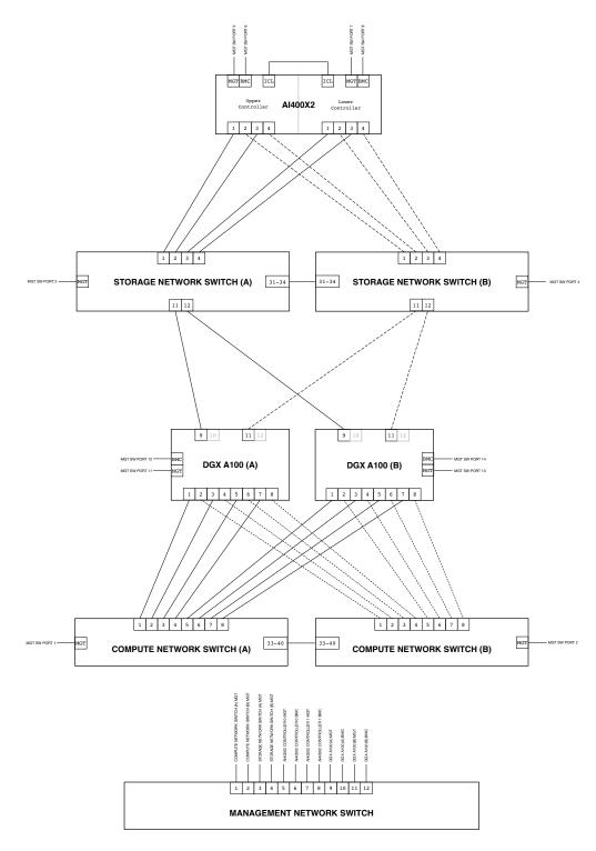
Figure 12. DDN A<sup>3</sup>I POD network diagram with two DGX A100 systems.
