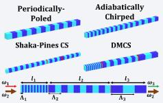
We show a proof of concept for implementing DMCS schemes in SFG QPM crystals and demonstrate its superiority over other common QPM schemes under length and power constraints.
