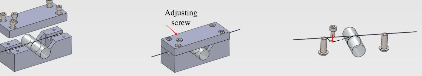
An adjusting screw, when fastened, "pushes" the tapered fiber toward the disc resonator, changing the effective coupling length.
