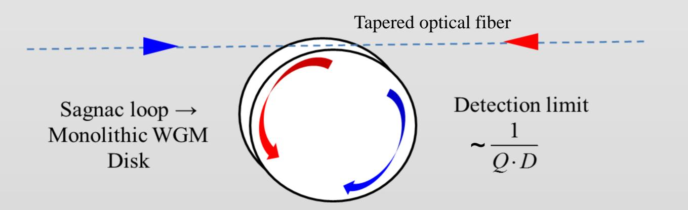
In FOGs – length serves for high angular velocity sensitivity. Here, the effective **long lifetime** of the optical mode inside the resonator alleviates the need for long distance phase accumulation.
