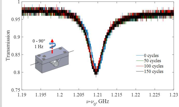
The robustness of the device was examined by rotating the entire construction back and forth  $\pm$  45 degrees at a frequency of 1 Hz.
