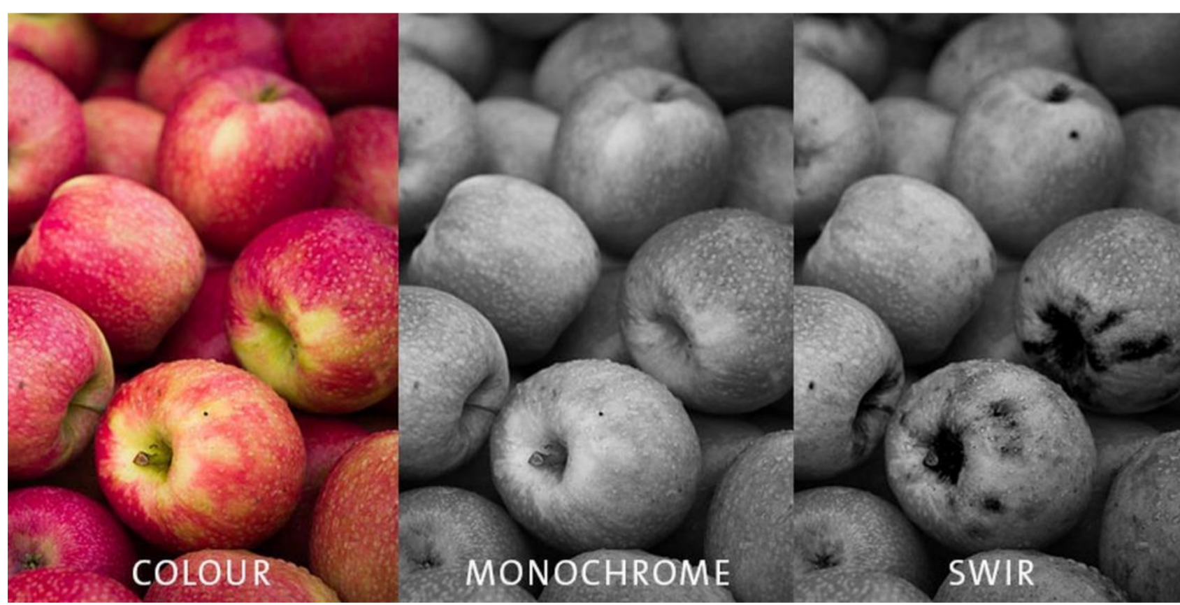
Figure 2 – SWIR application example, images of the same apples in different spectral ranges. 1
