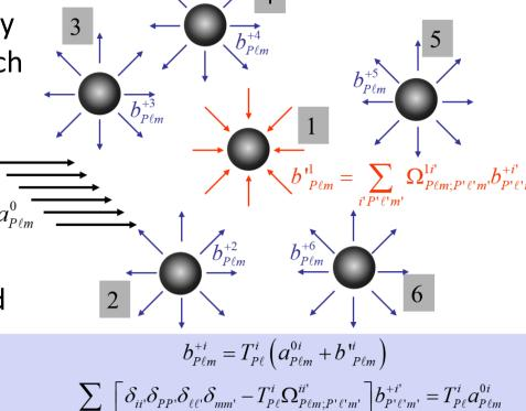
The Dynamic LMS is semianalytical and fast, (few seconds on a laptop), and allows the efficient design of dynamic metasurfaces
