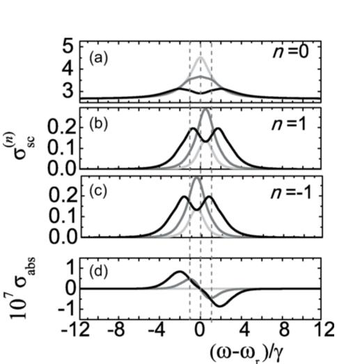
Fourier components of the optical scattering and absorption cross section, for the first-order  $TE_{\ell}=12$  Mie resonance
