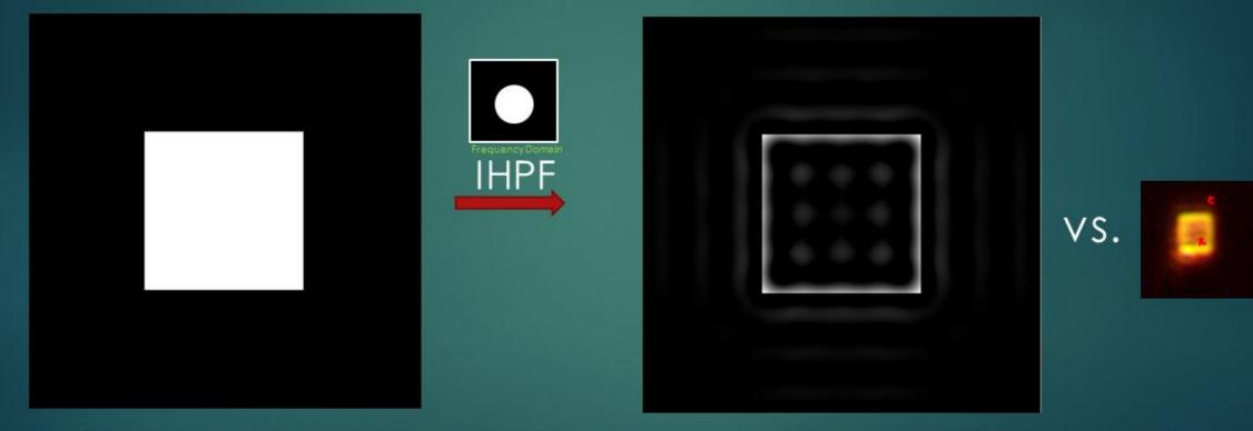
A simple computation using an Ideal Hi-Pass Filter (IHPF) reproduced the essential characteristics of the measured images.
