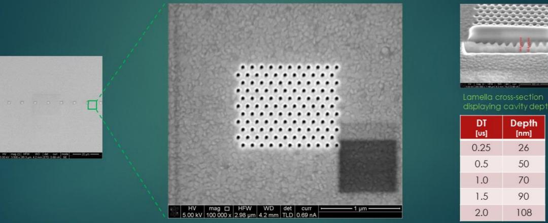
A series of such patterns were created at increasing depths, parameterized by the ion-beam dwell-time. Using SEM imaging, depths were determined to span the range 25-110nm.
