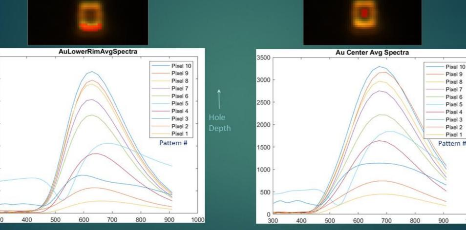
No significant difference in spectra was observed between the bright perimeter and the dark interior  $\Rightarrow$  the frames are not due to an excitation localized on the perimeter.
