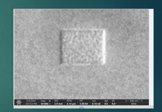
'Control patterns' were fabricated to test this - empty rectangles exposed uniformly to a low-dose ion-beam.
