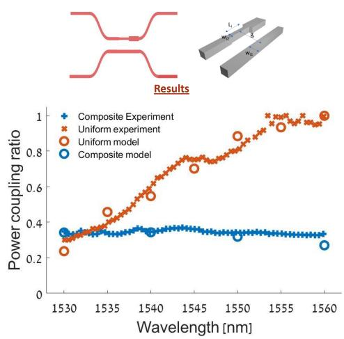
Power splitting ratios of the two couplers as functions of wavelengths. The splitting ratio of the long, uniform coupler varies between 0.3 and 1, whereas that of the composite-sections coupler remains within 0.34  $\pm$  0.02. The results illustrate the superior robustness of the composite-sections design with respect to wavelength changes. Agreement between models and measurements of splitting ratios is very good.
