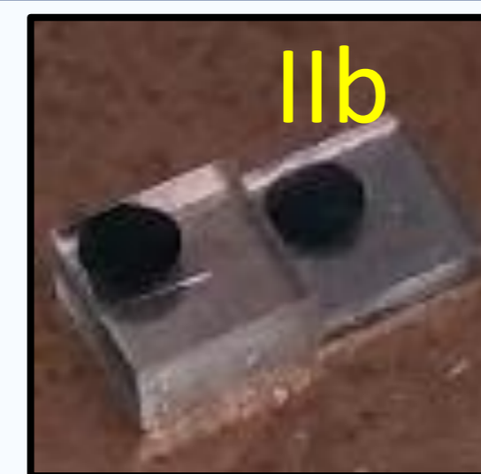
Ni-implanted <111> diamond samples
