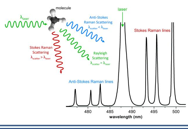
Raman spectroscopy: The laser focuses on the sample, causing a small portion of scattered photons to lose energy, which is absorbed by the molecule's vibrational energy levels. By using a spectrometer to measure the shifted photons (with altered wavelengths after filtering out the original laser light), we can obtain a spectral fingerprint of the molecules, with intensity reflecting their density.
