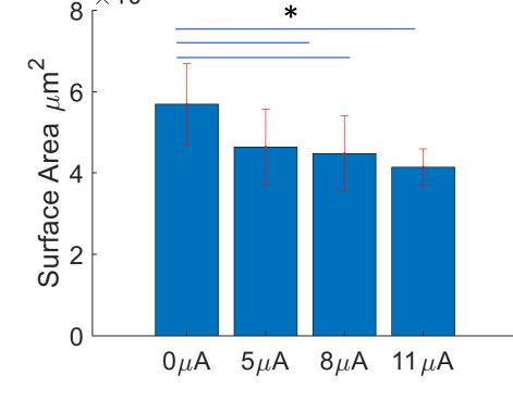
Opposite polarity current injected in the surrounding electrodes with increasing amplitudes resulted in confinement of the spatial spread.
