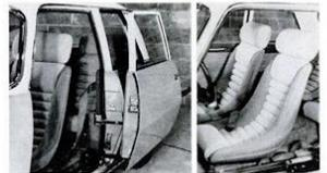
**DOORS AND SEATS.** Futuristic Italian car has safety doors that slide back on runners and won't fly open on curve. Lightly padded Italian four-seater seats have rock rests to keep a passenger's back from snapping back.
