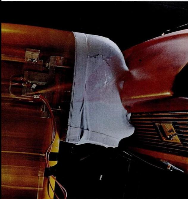
**DASHBOARD TEST.** A dummy skull made of rubbery plastic crashes into dashboard of Ford's Deanevan testing grounds to simulate a passenger's head being thrown violently forward in a collision. Instruments behind skull measure impact. Dash is covered with thick plastic padding being tested to measure its ability to prevent laceration and absorb impact.
