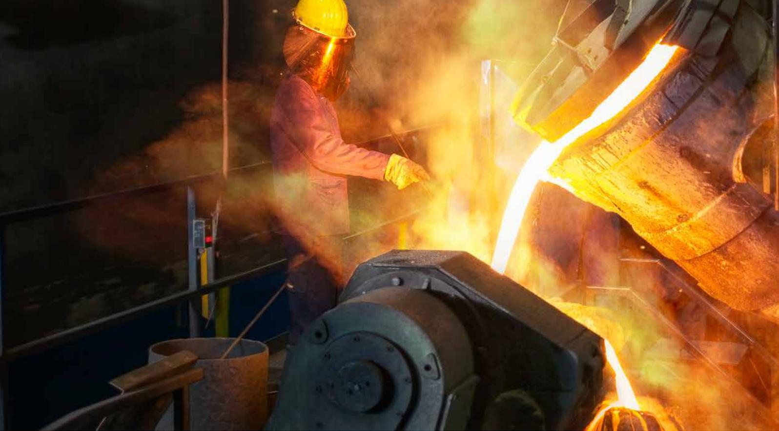
Filling the centrifugal casting machine
