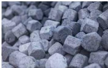
Silicon carbide to increase the silicon content in the iron
