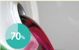
Water-glycol fire-resistant hydraulic fluid (70% share in Japan)
