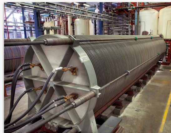
Alkaline electrolyzer stack
