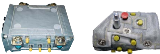
( 8 ) ISOLITE-Blanket (non-metallic) FADEC Box and Hydraulic Main Gear Control Valve
