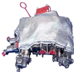
( 4 ) ISOLITE-Blanket Thrust Reverser Actuator
