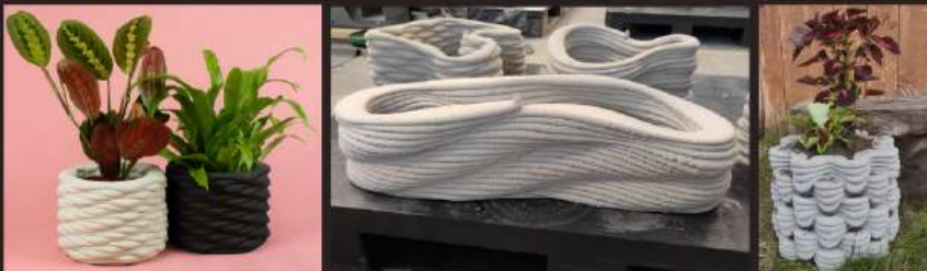
Concrete Planters - Non-Planar Printing; Color Printing
