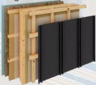
1. Construction of the external load-bearing wall
