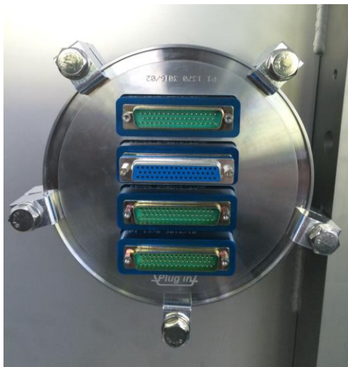
Figure 3. Four Sub-D connectors (50 pins) for data acquisition
