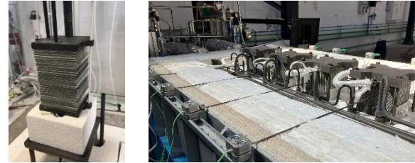
kW range co-electrolyser for hydrogen production or CO<sub>2</sub> methanation
