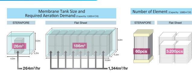
STERAPORE: 2,400m2/module × 1 module = 2,400m2 @ Flux 26 LMH : 320m²/module × 8 module = 2,560m² @ Flux 24 LMH
