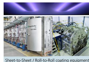
To bring the technology into relevant dimensions the up-scaling to pilot-scale industry level by large area magnetron sputtering and inline flash lamp annealing has been investigated and demonstrated.
