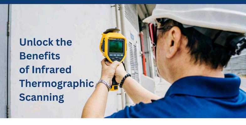
At R.A.K. Materials Consultants Pte. Ltd., we harness the cutting-edge power of infrared thermographic scanning—a non-contact method that identifies temperature variations in walls, beams, and ceilings. This innovative approach allows us to pinpoint potential issues without any physical contact, safeguarding the integrity of your property.
