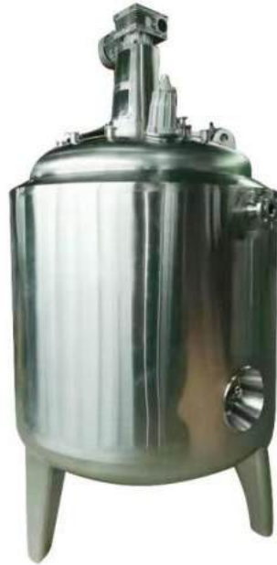
100L Reactor Water + Catalyst 200°C
