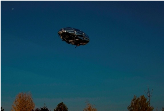
KUZGUN_1 All Electrical Unmanned Airship (completed)
