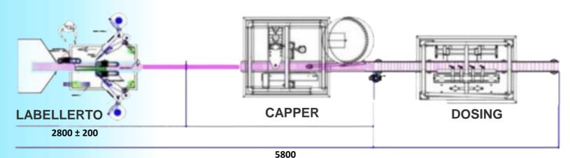
Labellerto apply label and back label on cylindrical, flat containersor oval. Made of stainless steel, Label positioning control via touch screen. It has a label breakage alarm, end of labels, real-time average production calculation. Adaptable to different container sizes...
