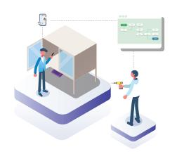
4. After the request; the user who has finished with the tool replaces the tool in the ISL. The second user who has requested the same tool opens the ISL with the RFID card and takes the tool. The same process as step 2 is repeated
