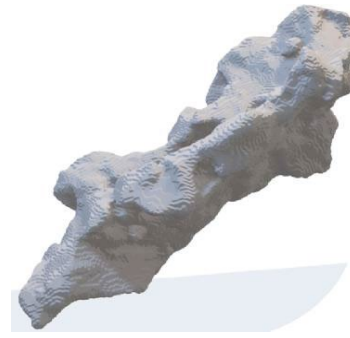
Figure 1. Regolith particle generated by 3D X-ray Tomography at TUBAF. The length of the particle is 240 \mu\text{m} .
