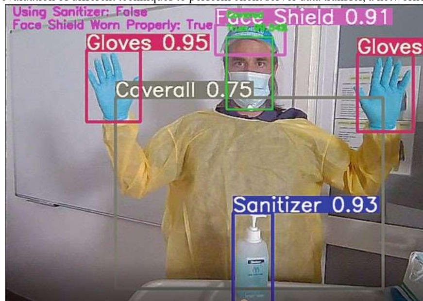
Fig. 7.4 Correct face shield wearing validation
