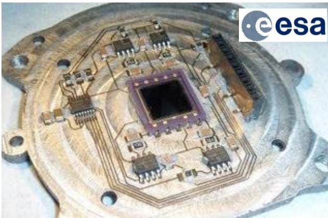
Housing of sun sensor. Printed electronic on the surface. Aluminium
