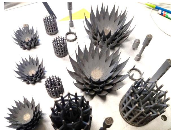
Heat sink designs developments for lamp Aluminium
