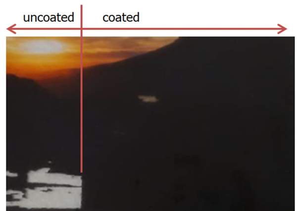
Picture 4: Much better adhesion on coated glass
