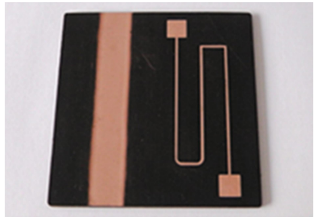
Picture 1: Structured conductive layer on composite
