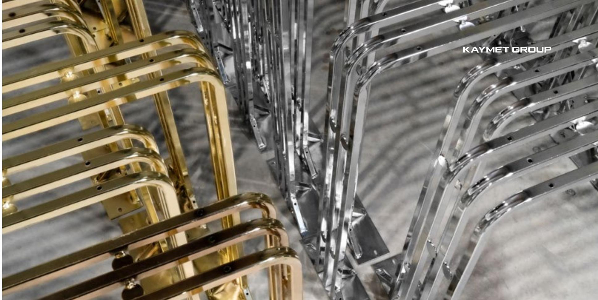
As Kaymet Metal, we have completed with the polishing and chrome facility we invested in in 2019 of the special surface coating materials that we specialize in supplying throughout Turkey. To meet the increasing need for high-quality coated semi-finished products especially in the store decoration, shelf and furniture industry, we introduced our 4-station, fully automatic polishing machines and semi-automatic chrome/nickel-plating facility with a coating capacity up to 600-1000 mm to the market.
