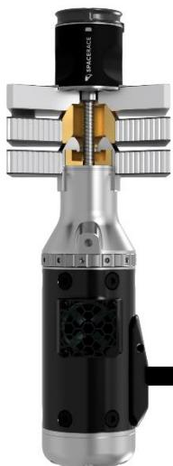
The UNIKA tensioning device is designed for applications up to 50 kN. Typical use is for preload of **Hold Down and Release Mechanisms** on spacecraft solar array or other deployables. Preload is achieved electronically by controlled heating of the Shape Memory Alloy.
