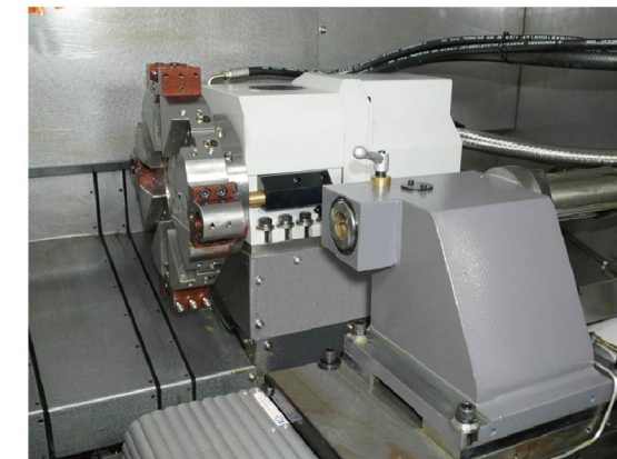
The Standard servo turret gives a accurate and speedy tool change. The hydraulic programmable tailstock with 150 mm manual stroke.
