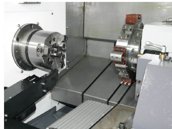
The Jaw chuck with gantry turret: The jaw chuck of 5" and 6" optional give the cutting range more flexible.
