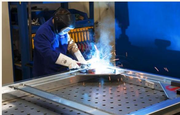
**Conventional Welding:** sheet metal and structural manual welding MAG (135, 136), MIG (131), TIG (141) using **Fronius** and **Lincoln Electric** machines, various materials and thickness
